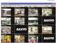
Dedicated software for recording, playback and monitoring of video feeds from a multiplicity of surveillance cameras.
